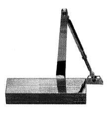
Gainsborough 3100 Series Hydraulic Door Closer. Compact design with minimal projection, for internal or external doors. Standard backcheck with regular and parallel arm installation and power adjustment.
